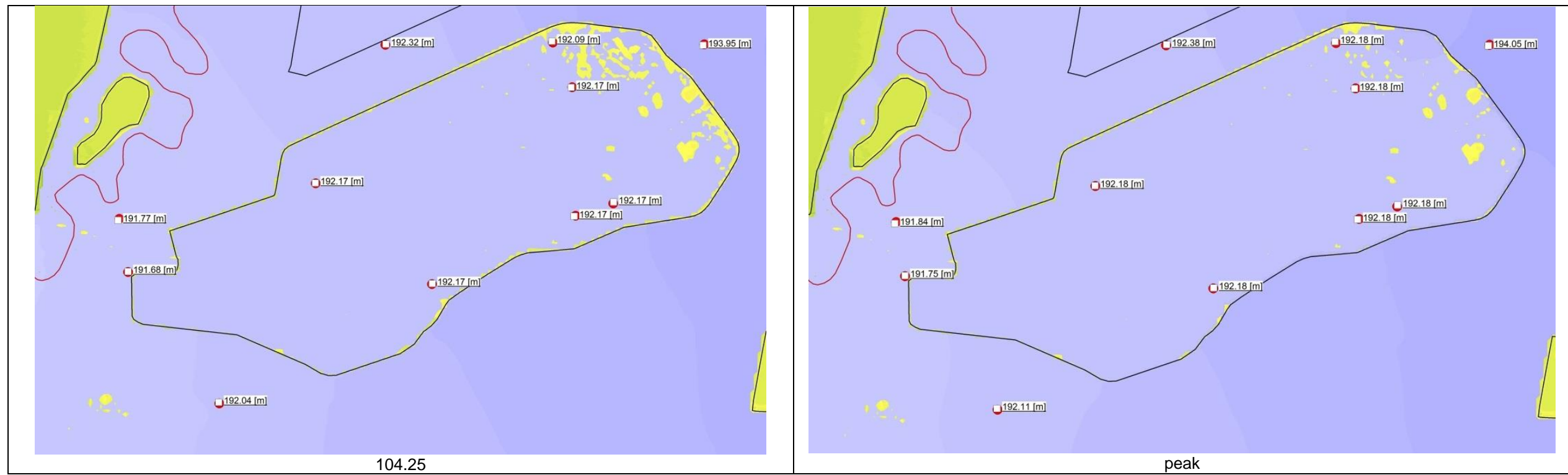
Figure Appendix D-3 Progression of flooding through Wee Waa when the levee is overtopped during a 1% AEP design flood event
