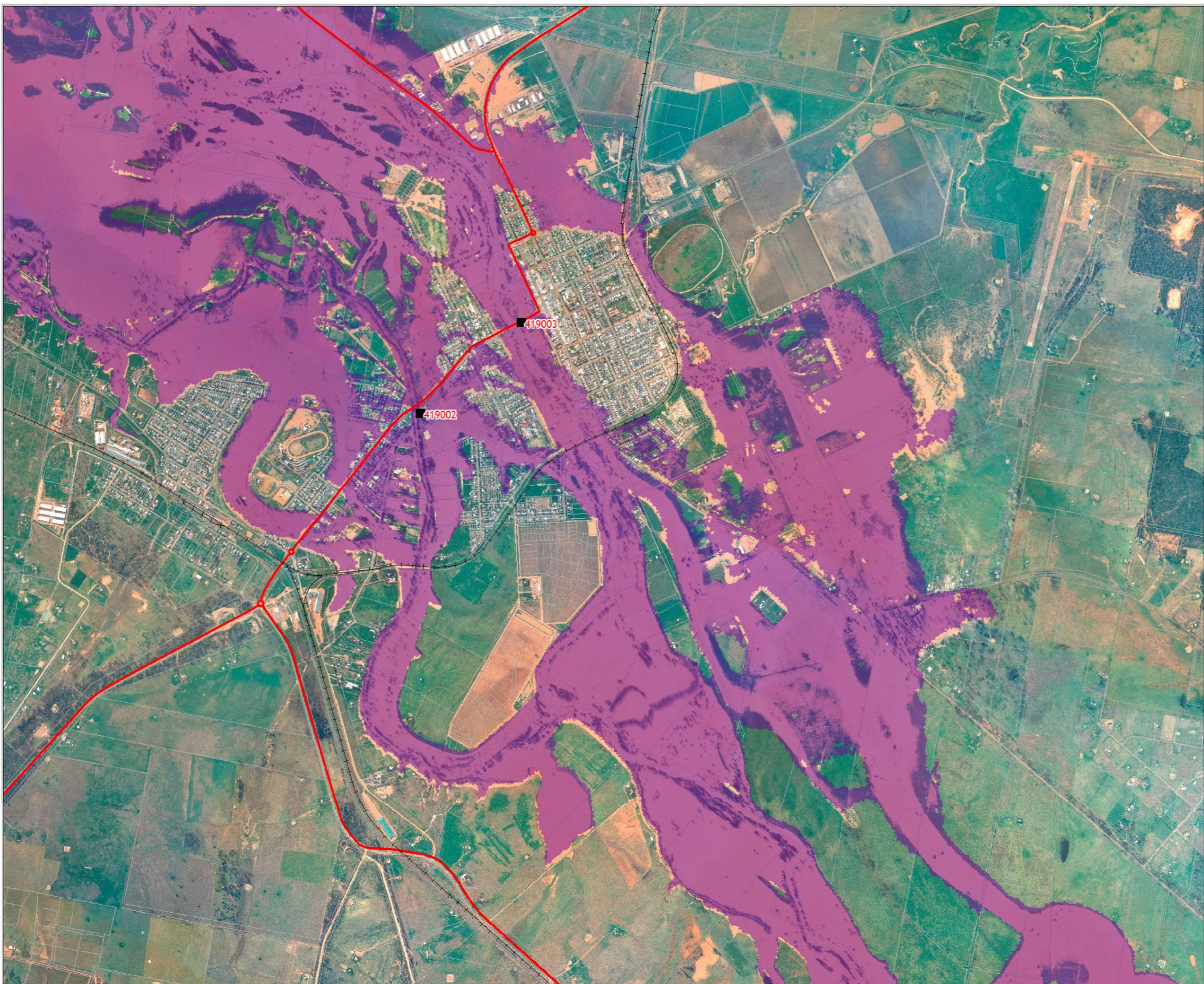
Figure A.4: Predicted and Observed Flood Extents July 1998
